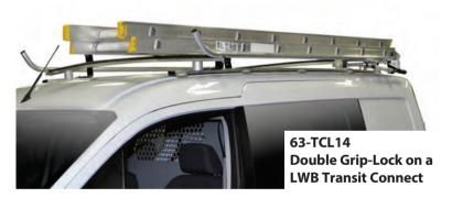
\*Note: This rack can accommodate 28 ft. extension ladders with extra length extending off the rear of the vehicle for balance. Check with local regulations regarding rear overhang of loads.
