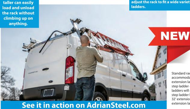
Standard rack accommodates 28' extension ladder and 10' step ladder – short step ladders will need optional step ladder kit and up to 32' extension ladder with extension ladder kit.
