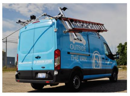
**DDLR61FTM** - Single, Transit Medium Roof **DDLR63FTM** - Double, Transit Medium Roof
